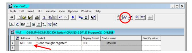
Note: It's possible to choose any of the weight registers listed below, the chosen weight register will show at address PID 256 (weight register).
