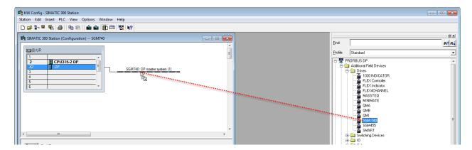
Set the Profibus address of the SGM740 or SGM840 (the same address as used in Pi Mach II) and click on **OK**. See <u>Setup the SGM740 or SGM840</u>.
