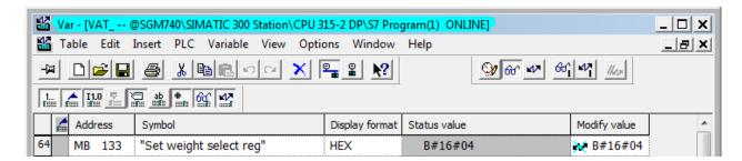
To check if the SGM740 or SGM840 has executed the weight select register, it's possible to read out the weight select register. Please see <u>Read weight select register</u> for instructions.
