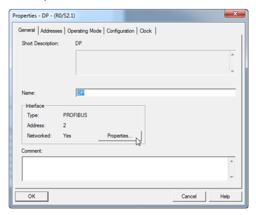
Set the Profibus address for the PLC and click on **New** to set up a Subnet.
