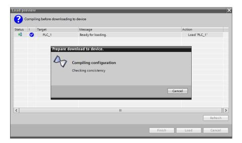
Click on Load to download the configuration into the PLC. When completed click on Finish.
