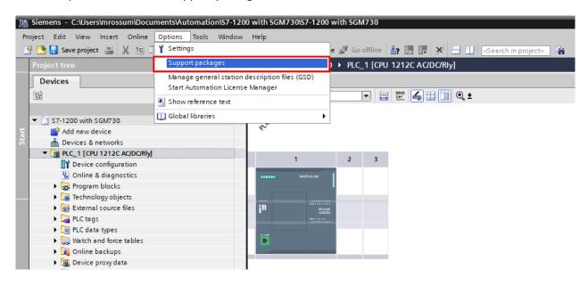
Select the HSP0079 S71200 CANopen file and click on Install. If it is not shown, click on Add form file system and locate the file. When installed, click n Close.
