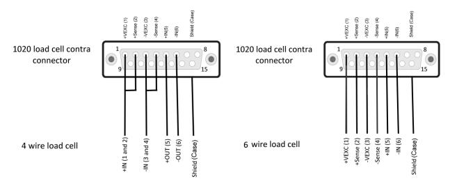
Note: when you use a 4 wire load cell, +IN <u>must</u> be connected to +VEXC <u>and</u> +Sense. –IN <u>must</u> be connected to -VEXC <u>and</u> -Sense.
