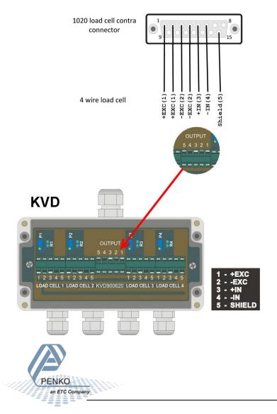
PENKO How to... Connect up to 4 load cells to the 1020
