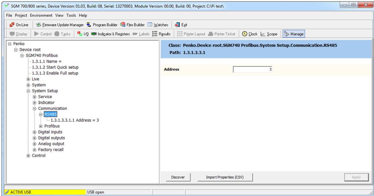
If all addresses are set, connect the device with address 1 to the PC with a USB-cable or Ethernet cable if available.
