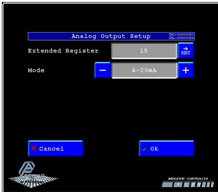
In the example above the **Extended Register** is set to Register 15 and the **Mode** is 4 – 20mA.
