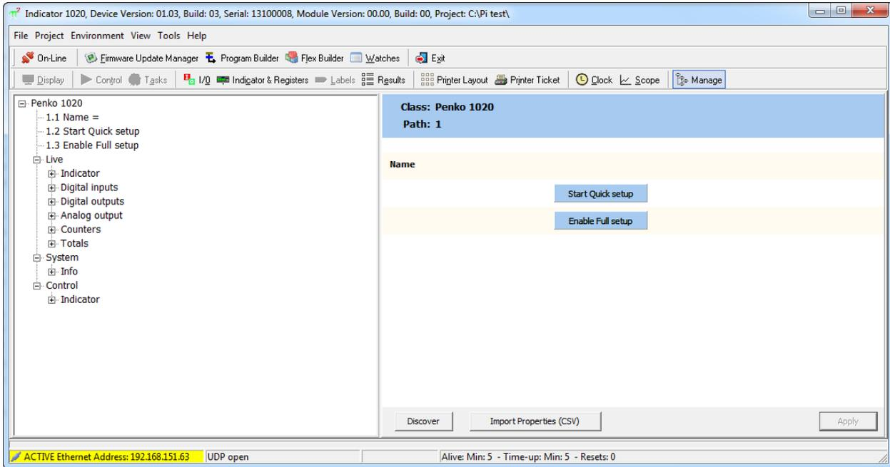
Click on **Enable Full setup** and double click on **System Setup**, then double click on **Analog outputs**, double click on **Configuration**. Here you can change the following parameters:
