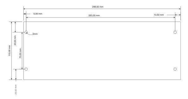
Unit size is 298,5x110x120mm (hxwxd).
