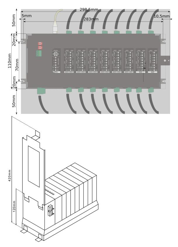
Allow for room for the front brace which hinges up to 300mm in front of the unit.
