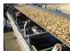
Photo 3. A continuously totalising belt weigher.
