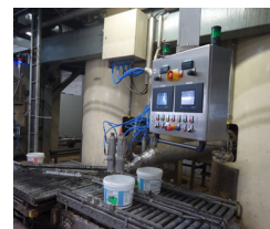
Photo 1. A gravimetric filling installation.
