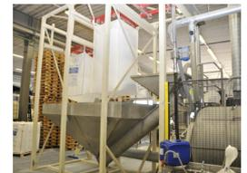
Photo 3. The intake of raw materials into the process out of big bags.
