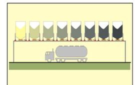
Figuur 10. Filling a truck by means of weighing silos.
