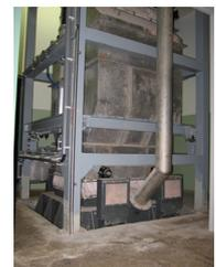
Photo 7. An installation for the discontinuous totalizing loading of bulk material.
