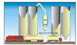
Figure 12. Filling a truck via a mobile belt conveyor.
