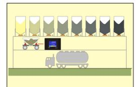
Figure 11. Filling a truck by means of a mobile weighing hopper.
