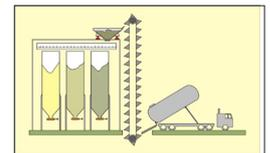
Figure 2. Receiving raw materials by truck.
