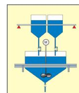
Figure 9. A combined weighing frame for the liquid ingredients.
