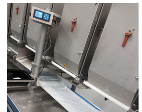
Photo 4. An example of a weighing platform for dosing small quantity components manually in advance.
