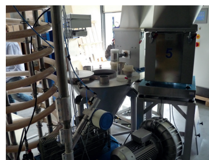
Photo 1. A weigh hopper for negative dosing.
