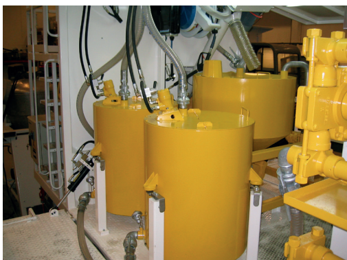
Photo 2. The continuous preparation of a mixture out of three weighing tanks.
