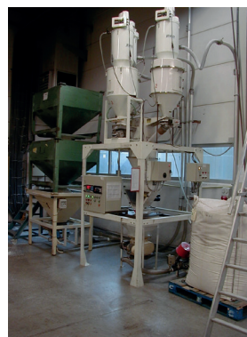
Photo 3. The realization of a continuous flow out of two weighers.
