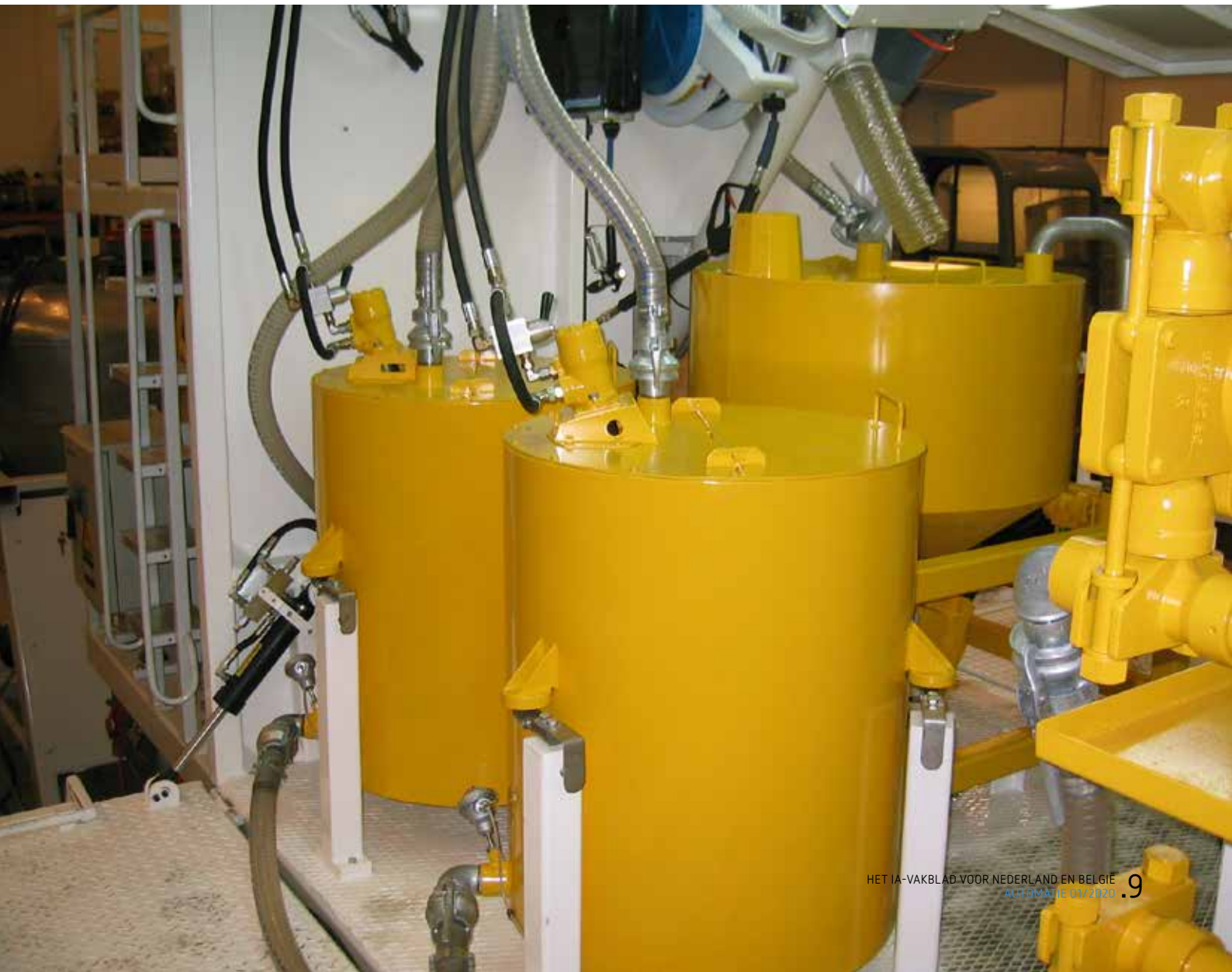
▽ Photo 2. The continuous preparation of mixtures out of two liquids and two solids
