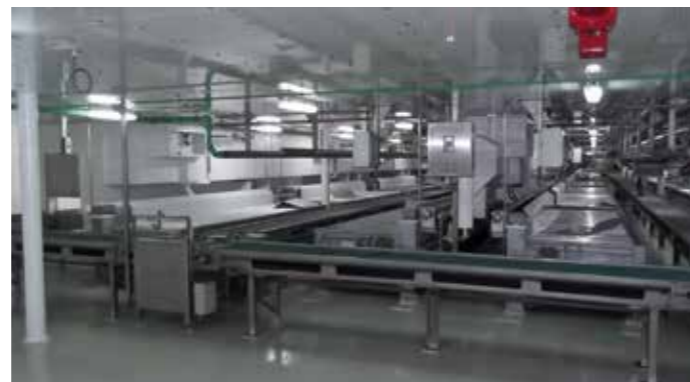
One of the weighing belts, built by Afak and equipped with Penko weighing technology
