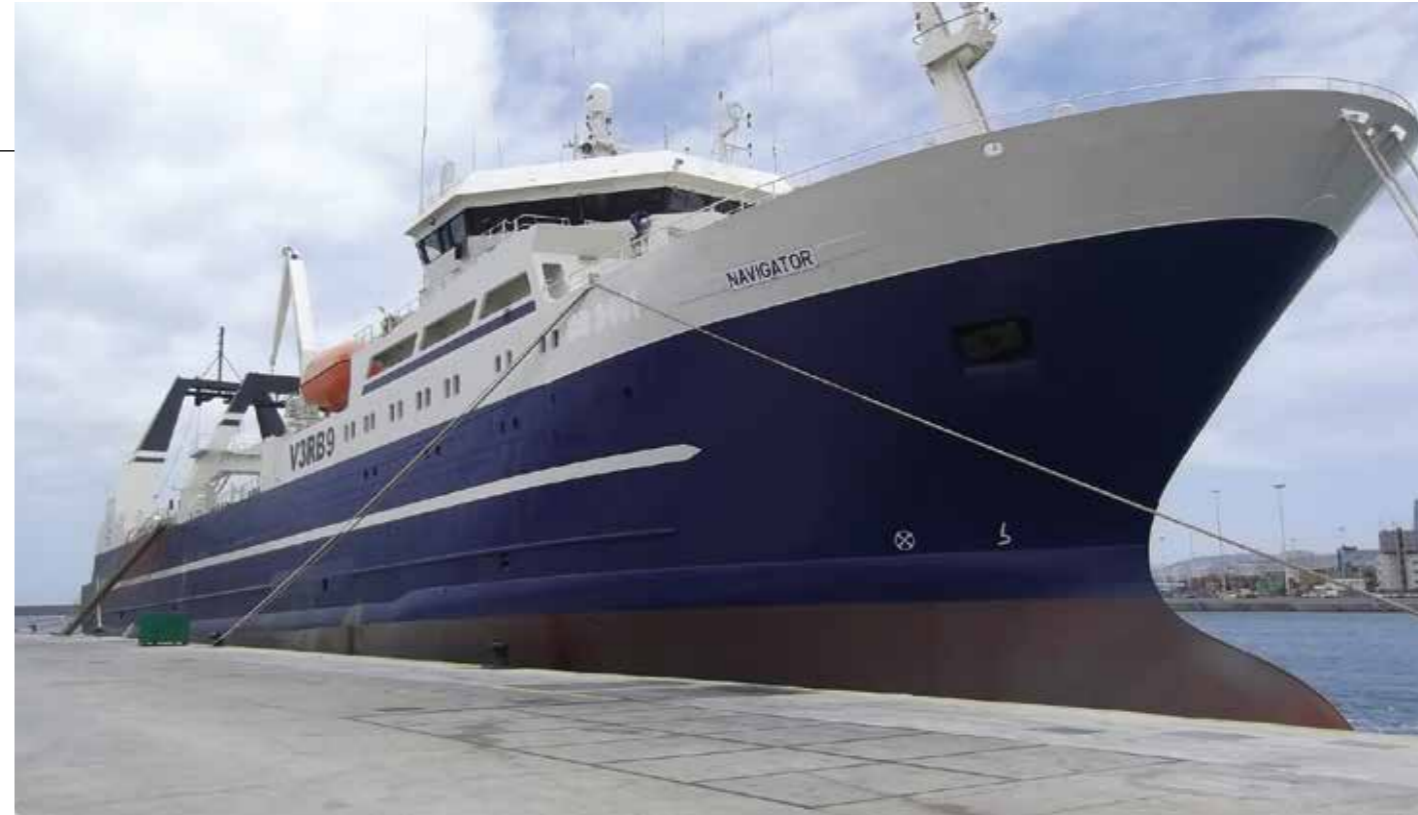
The Navigator is a factory trawler with a length of 121 meters and a loading capacity of 4065 metric tons
