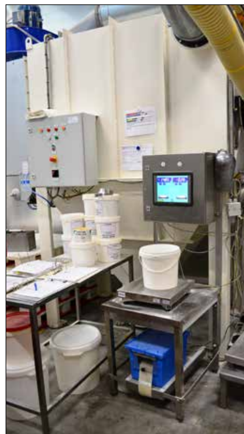
The automatic recipe dispenser with software from Penko Engineering includes a tray for weighing in kilos and a tray for weighing raw materials in grams; it is very user friendly
