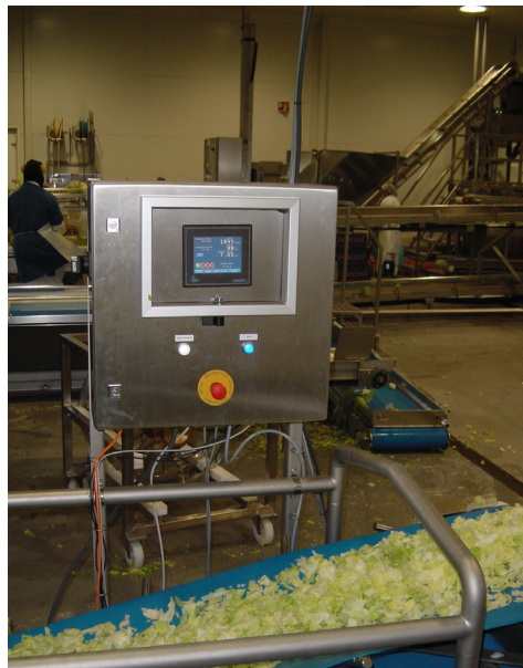
in spite of the relatively high mass of the belt conveyor a system with a weight controller could be realized.
