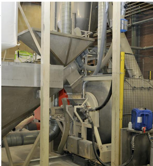
The second process, which is largely a dry process, consists of spraying an acid blend onto a carrier which is typically a powder (? yes). First the powder is dosed from a big bag into an interim intermediate (?) hopper
