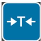
T Starts the dynamic zero level measurement. During this measurement the average weight of the empty belt is determined
