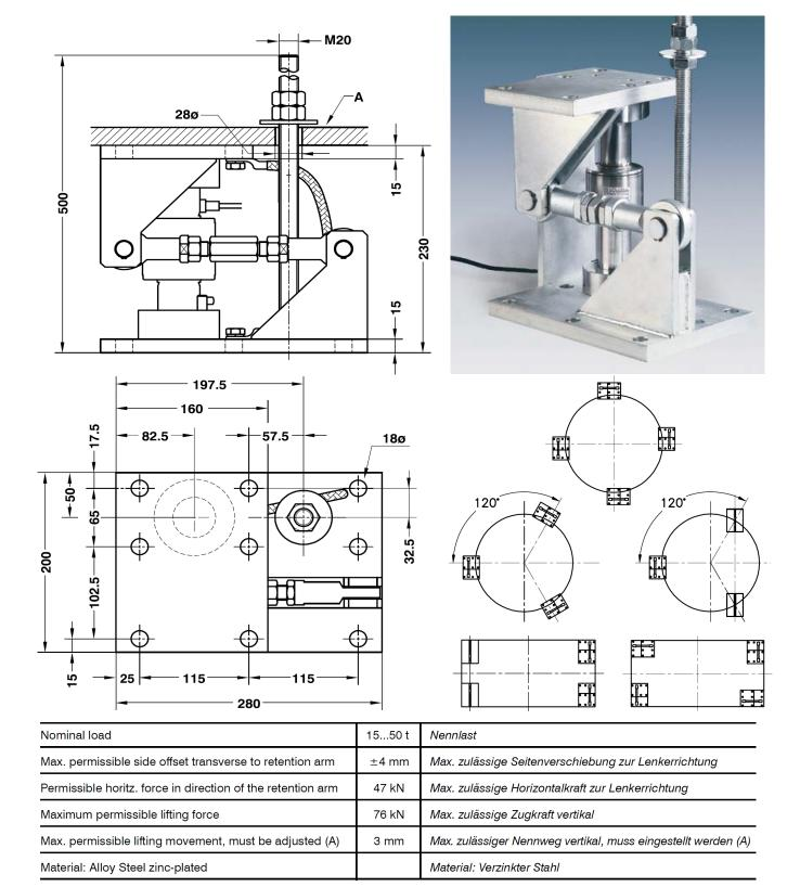
Dimensions in mm. Abmessungen in mm.
