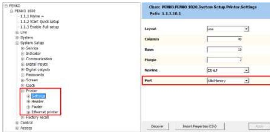
Every time the Print button is pressed, a new alibi record is created. To see the alibi record, go to the Access menu and select Alibi.
