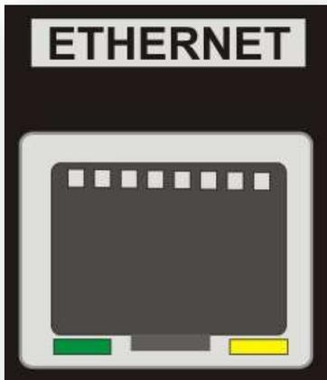
The Ethernet connection can be used for communication with Pi Mach II and for the following protocols:
