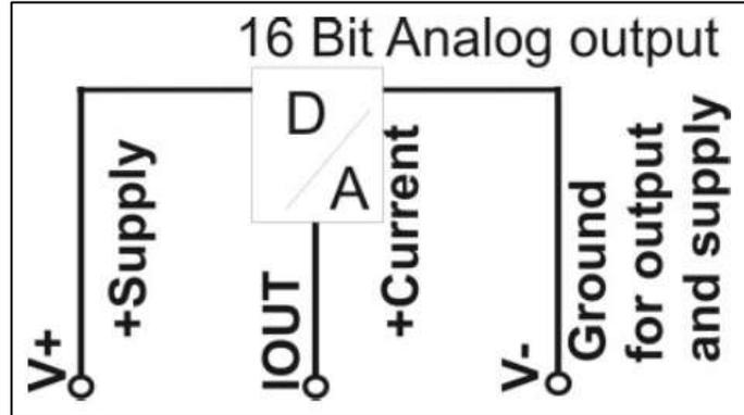
The analog output can be used as mA output in the following ranges and react to an indicator value.
