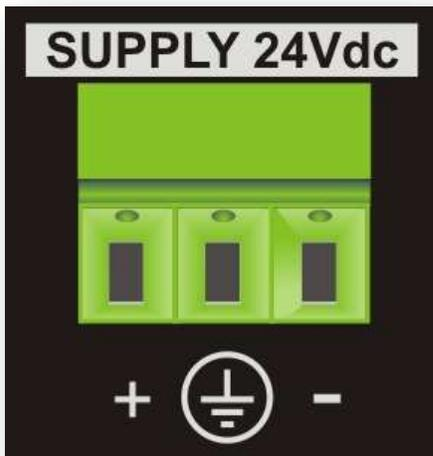
Power the device using a Class 2 or Limited Power Source, rate 18 – 32 VDC, 0.4A@24VDC
