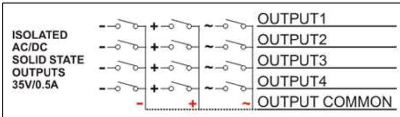
The device has 4 digital outputs that can be used for an AC and DC power circuit up to 35V/0.5A.
