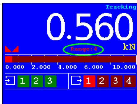
In multi-range mode, the range will only get back to range 1 when the indicator has been lower or equal to zero. In this case, when the value goes down, range 4 will remain active until the indicator reaches zero.
