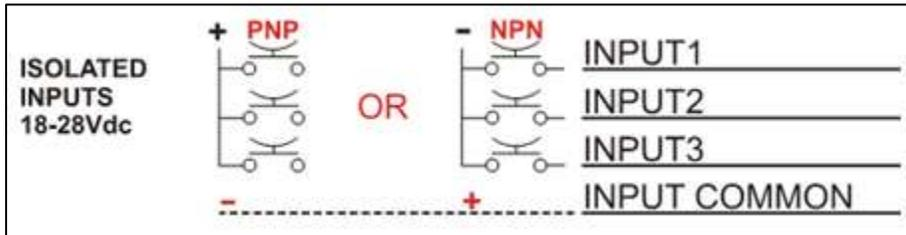
The device has 3 digital. The inputs can be switched PNP or NPN with 18 - 28 VDC.
