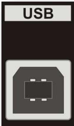
Connect the device to a computer using an A-B USB cable. The USB interface is used for communication with PENKO configuration software.
