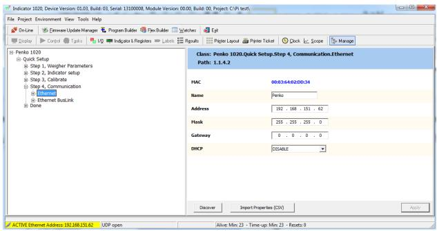
The standard 1020 only has Ethernet, but if you have a Profibus or RS232/RS422/CAN bus option board these parameter will appear at step 4 (Communication).
