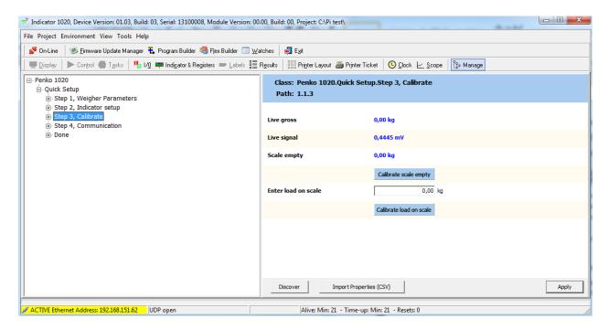
Make sure the weighing installation is empty. Click on Calibrate scale empty.
