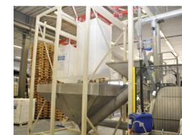
Photo 3. The intake of raw materials into the process out of big bags.
