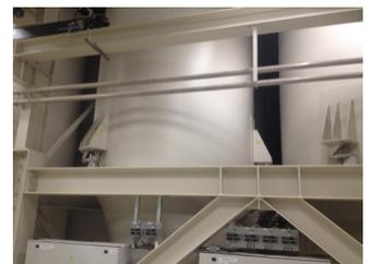
Photo 6. Weighing silos for the storage of finished products.
