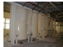
Photo 2. The silos for the interim storage of incoming raw materials.
