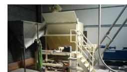
Photo 4. A cabinet for the manual addition of raw materials.
