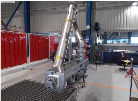
A weighing screw at the Van Beek plant, showing (right) the control panel.
