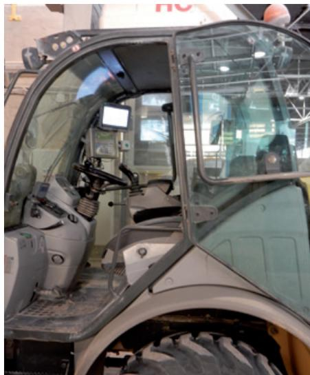
Fig. 3 De shovel with the operators-terminal
