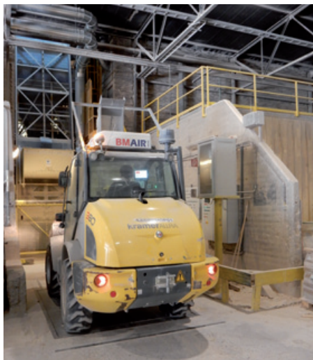
Fig. 2 The lift truck on the floor scale to determine the tare weight
