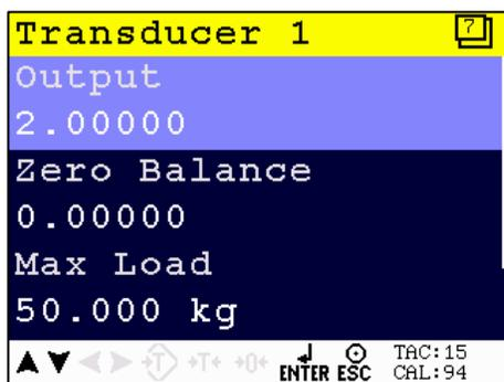
*Output, zero balance and max load are calculated from TEDS information*
