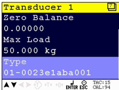
*01 indicates this TEDS load cell is connected to input 1*
