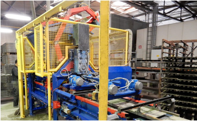
Hardening spacers Discharge of concrete in the moulds
