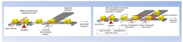
**Note:** these combinations of belt conveyors belt can also be used, optionally without pusher(s) for class Y applications.
