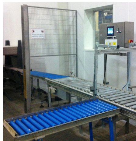
Fig. 3 A checkweigher with ejection system
