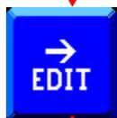
Press "EDIT" and put a reference weight on the weigher. Enter the weight of the reference weight and press OK.
