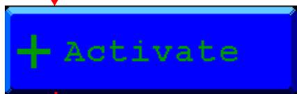
Make sure the weigher is empty and press the "+Activate" button to save the zero point
