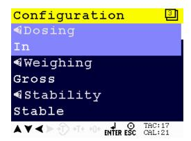
When pushing the LEFT key, the help text of the parameter is shown. Below the example for of the help text for the parameter Dosing.
