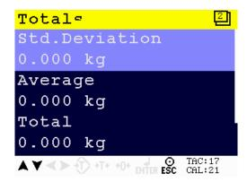
Totals and subtotals can be printed by pressing Enter.
