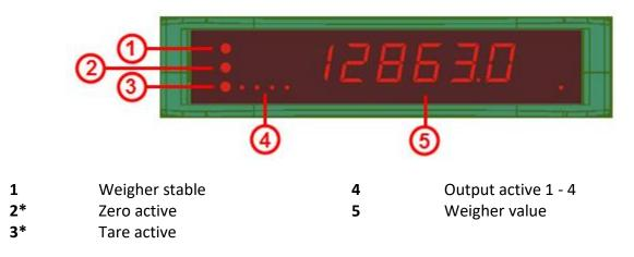
\* When the check weigher program is active, LED 2 and 3 are blinking
