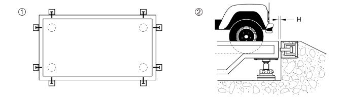
Using accessories **75903** + **75905** the platforms admit the use of tie rods or stoppers. If stoppers are used ① it must be left a maximum spread ② of: H<6 mm. We recommend to clean and to grease periodically the joints.
