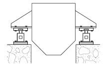
The upper support **72906** - **72907**, has a high hardness plate to avoid load cell damage. This accessory is suitable for structures that has not to support important dilation or lateral forces.
