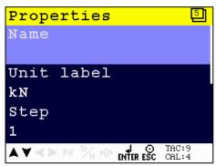
Here the Unit, Step size, Decimal point and Max load can be set
