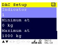
Scroll through the DAC Setup menu using the UP or DOWN key. Press Enter for editing the setting.
