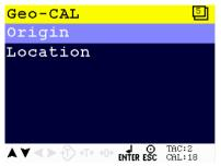
Scroll through the Geo-CAL menu using the UP or DOWN key. Press Enter for editing the setting.
