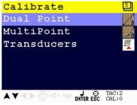
Scroll through the Calibrate menu using the UP or DOWN key. Press Enter for editing the setting.
