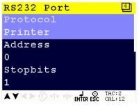
Scroll through the RS232 Port menu using the UP or DOWN key. Press Enter for editing the setting.
