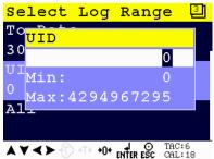
Use the UP, DOWN, LEFT and RIGHT key to enter the UID code. The UP and DOWN keys
