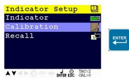
Enter CAL (number) by using the UP key and confirm with Enter.
