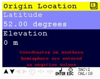
Scroll through the Geo-CAL menu using the UP or DOWN key. Press Enter for editing the setting.
