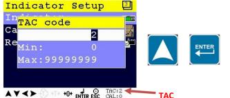
**TAC** TAC (Traceable Access Code) shows on lower right of the screen. Every time settings are changed, the TAC automatically levels up by 1. Example TAC:2
