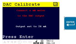
Use the UP, DOWN and LEFT key to enter the reference value. The UP and DOWN keys are used for changing the number (1-9), the LEFT key is used for changing the position of the cursor. Confirm with Enter.
