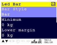
Scroll through the Led Bar menu using the UP or DOWN key. Press Enter for editing the setting.
