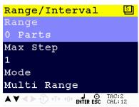
Scroll through the Range/Interval menu using the UP or DOWN key. Press Enter for editing the setting.
