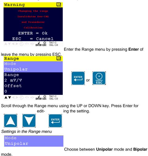
In Unipolar mode the input range for load cells is 0 mV/V to + selected value in mV/V.
