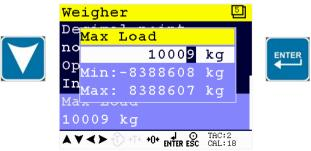
The max load prevents overload by user. Any weight above this set value will not be shown. If there is an overload, display shows the error code ======. *Note: In certified mode the max. load is not allowed to be more then the maximum load* + 9 scale parts.
