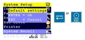
Starting at firmware version 1.5.0.9.0.3 a backup of the device configuration can be made within the device.
