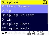
Scroll through the Filter menu using the UP or DOWN key. Press Enter for editing the setting.
