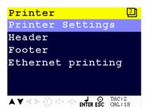
Scroll through the Printer menu using the UP or DOWN key. Press Enter for editing the setting.
