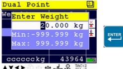
Use the UP, DOWN and LEFT key to enter the reference value. The UP and DOWN keys are used for changing the number (1-9), the LEFT key is used for changing the position of the cursor.
